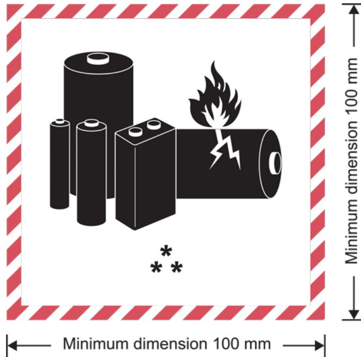
\* Place for UN number(s), i.e. UN 3090, UN 3091, UN 3480 and/or UN 3481, as applicable. The UN number(s) indicated on the mark should be at least 12 mm high.
